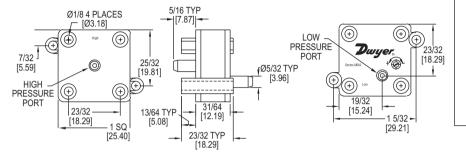
Series MDA Miniature Adjustable Pressure Switch is used to sense differential pressure. The switch features field adjustable set point and gold inlay contacts. The lightweight and compact size make the MDA ideal for any application with space constraints. Applications include industrial, HVAC, pump and motor control, medical, automotive, pools and spas.
