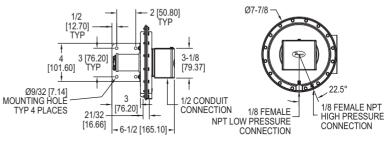
The unique electric switch design in the Series 1640 Floating Contact Null Switch for High and Low Actuation is another Dwyer Instrument, Inc. innovation. The Dwyer® Model 1640 Differential Pressure Switch resembles the high precision large diaphragm Series 1630 switches. However, the Model 1640 is equipped with a single pole, double throw floating contact switch (not snap acting) so it functions as a null switch.
